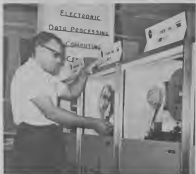
CHARLES LAMPE mounts tape reel in latest model tape units featuring glass panels which operate automatically.
